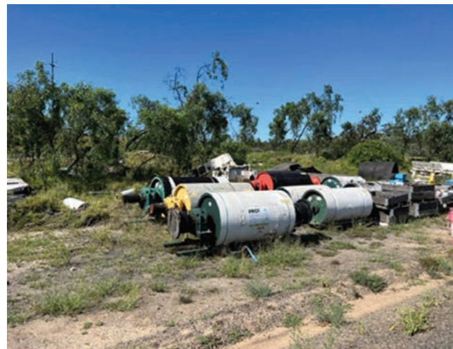
The above photographs illustrate the repurposing of second hand drive units which are proposed to be used for the conveyor systems in the Ironbark No. 1 mine development. These units were used and surplus to another coal mine operator's business. Again, this approach by Fitzroy generated work for the local community and repurposed existing equipment rather than importing new items
