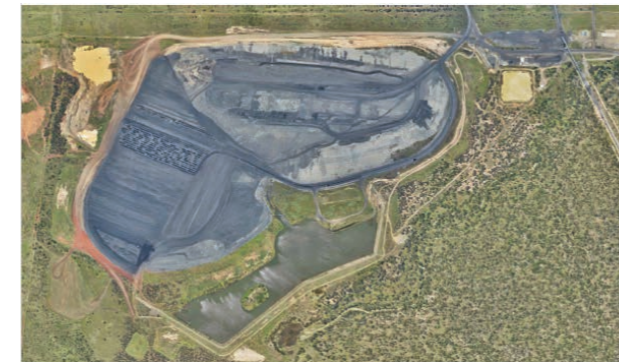
Note – no tailings dam onsite, all rejects material placed in Dry Rejects Emplacement Area.
