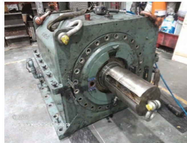
The above photographs illustrate the repurposing of second hand drive units which are proposed to be used for the conveyor systems in the Ironbark No. 1 mine development. These units were used and surplus to another coal mine operator's business. Again, this approach by Fitzroy generated work for the local community and repurposed existing equipment rather than importing new items
